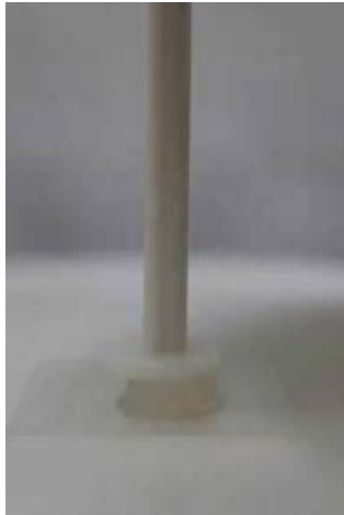
Regular gel with irreversible chemical crosslinking
