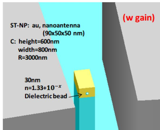
Fig. 2. Schematic of the active configuration. The micro-ring has a height of 600 nm, a gap width of 120 nm and an radius of 3 μm. The gold ST-NP is a nanoantenna. The detection is also dark-field spectroscopy in our simulation. The cavity is of optical gain doped. The environment is water ( $n=1.33$ ), and the target to sense is dielectric bead with  $n=1.33+10^{-x}$
