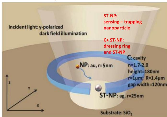
Fig.1. Schematic of the hybrid ST-NP configuration. The micro-ring has a height of 180 nm, a gap width of 120 nm and an outer and inner radius of 0.9 μm and 0.5 μm respectively. The silver ST-NP has a radius of 25 nm. The incident cone of light is used for dark-field spectroscopy.
