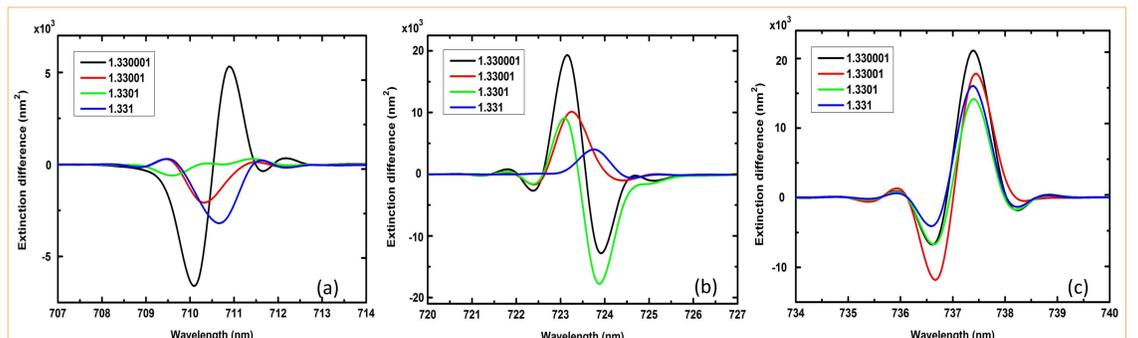
Extinction difference spectra (C+ST-NP+NP minus C+ST-NP) with the dressing ring of optical gain (Rh800). The target bead is of index varies from 1.331 to 1.330001.
