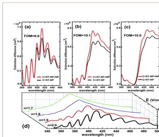
Evolution of extinction spectra of the C+ST-NP+NP and C+ST-NP systems with the refractive index of the dressing ring (a) 1.9; (b) 1.8; (c) 1.7; (d) near-field amplitude of the C+ST-NP system (data recorded by the point monitor).
