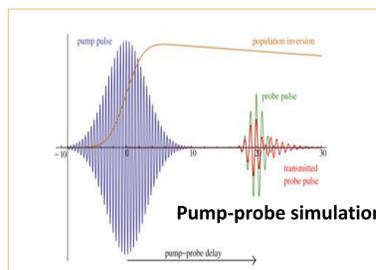
With gain in the ring, we use four-level two-electron model to simulate the solid Rh800 dye in epoxy.
