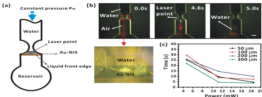
Fig. 2 (a) Schematic of valving operation driven by 785nm laser. (b) Temporal sequence of a 300 µm wide microfluidic valve (c) Valve opening time versus laser power for different valve.
