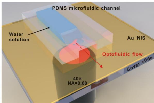
Optical setup of the experimental system
